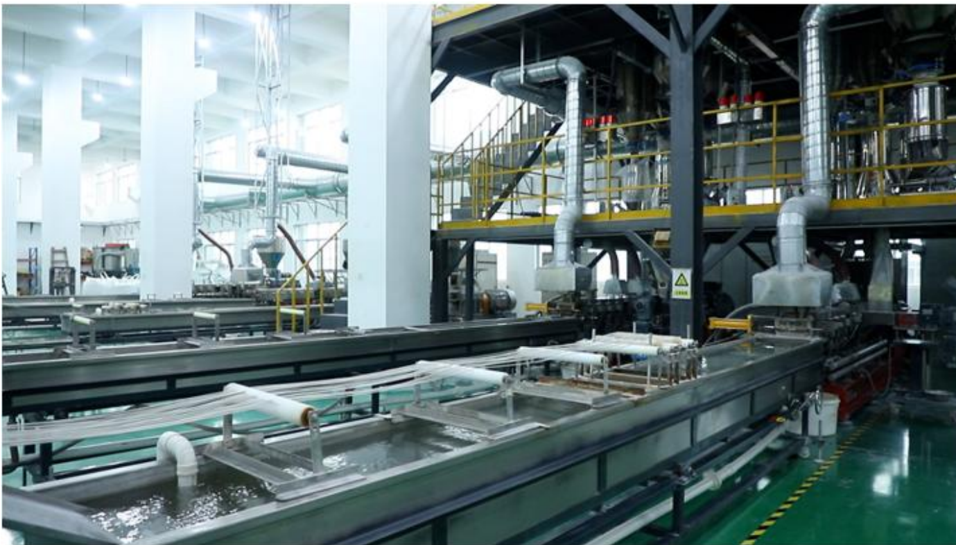
6 plastic pellet production lines with a capacity of about 1000 tons/month.
